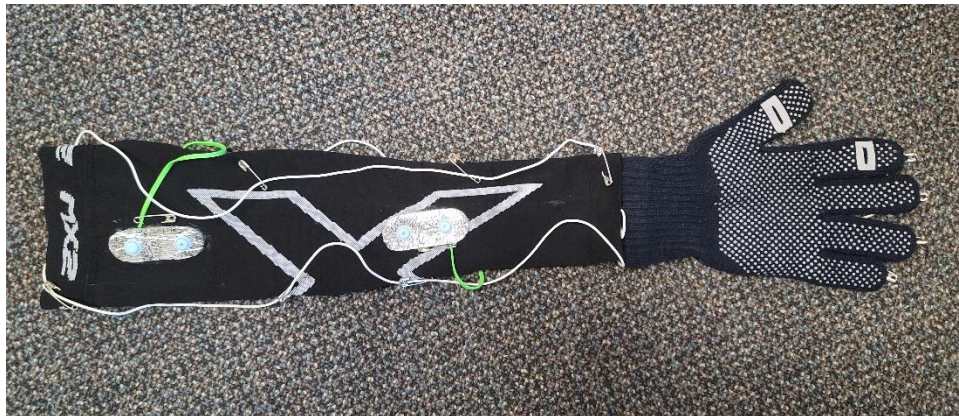
Figure 2: The medium-fidelity prototype (palm down), with heating wires and muscle sensors.
