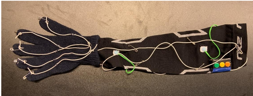
Figure 1: The medium-fidelity prototype (palm up), with heating wires and LEDs on top of the battery pack, located at the bottom right.
