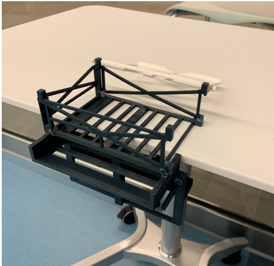
Figure 4: Raspberry Pi housing, the clamp is adjusted and customized to the thickness of the given surface.
